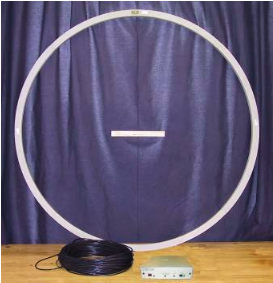
Assembled rotating transmitter with AT-4400 receiver and lengthy pickup-to-receiver coaxial cable.
