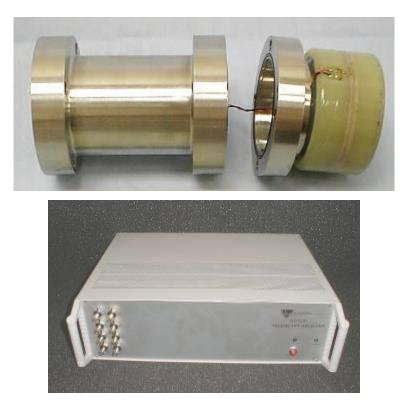
The picture above-left shows the Transmitter's electronics modular design for the 8 strain measurements; on the upper right, the electronics are shown in a rapid-prototype housing prior to insertion in a metal coupling. The exterior of the coupling, with a glass laminate induction power pickup coil assembly is shown in the lower left picture. The Receiver (digital to analog outputs device) is shown on the lower right.
