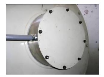
Figure 6 Diode Wheel Inspection Hatch Extension For Additional Clearance
