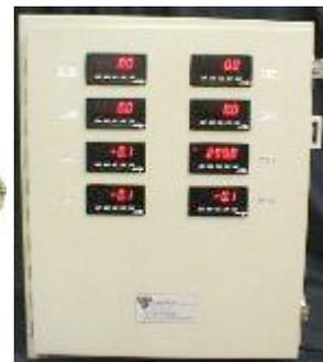
The above left picture shows the rotating Transmitter for the 8 RTD's (cover removed to show connections for the RTD's), the induction power/data coils (during testing in Schenectady) in the center, and the Receiver (digital to analog output device) on the right. The Receiver is equipped with optional panel meters providing  $y=mx+b$  unit translation (analog voltage to scaled temperature outputs).
