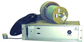
AT-7000 for Brake Temperature Testing 24 thermocouples, optical encoder, and rotary air pressure union
