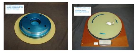
End of Shaft <u>AT-7000</u> system for monitoring 16 Strain Gages and 24 thermocouples (on a different generator) The AT-7000 multichannel system can measure RTD's, Thermocouples, Strain Gages, Pressure transducers, as well as differential Voltages (and Current shunts).
