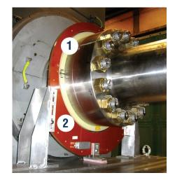
1 - Transmitter (Shown mounted on a 21.3" OD, 3000 RPM shaft) Rotating clamp-collar assembly supplying excitation to userinstalled strain gage and transmitting digital strain gage data to Pickup Antenna
