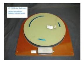
End of Shaft <u>AT-7000</u> system for monitoring 16 Strain Gages and 24 thermocouples (on a different generator) The AT-7000 multichannel system can measure RTD's, Thermocouples, Strain Gages, Pressure transducers, as well as differential Voltages (and Current shunts).
