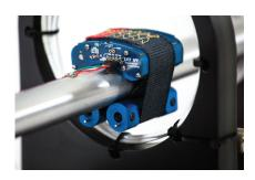
Need to take measurements for a temporary application or in small spaces? Our AT-5000 battery-powered digital telemetry systems are mounted to a shaft using a heavy-duty aramid fiber strap. It measures, digitizes, and transmits data wirelessly off rotating half shafts, drive shafts and rotors to a stationary receiver which converts the digital data to an analog output voltage. These systems are
