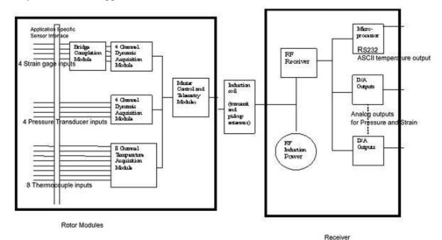
Once the data are digitized, the bits are organized for transmission in serial fashion. This organization must include provisions for synchronizing the receiver to the digitizing process. Usually "frame synchronizing" bits are combined with the data to allow the receiver to process the information appropriately. Digital data on a radio frequency
