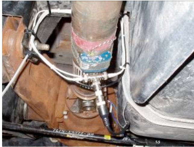
AT-5000 EasyApp truck driveshaft installation with Flexible Loop pickup
