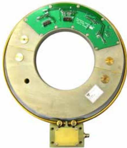
Split clamp-collar transmitter, multiple modules, epoxy-glass (G10) construction, and stationary loop coil
